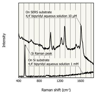
Integration time: 1 s, average count: 10 • When using SERS substrate: Laser intensity: 5 mW
