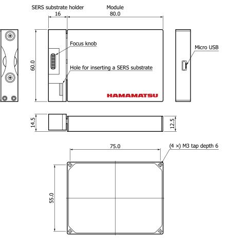
Tolerance unless otherwise noted:  $\pm 0.5$ Note: With the SERS substrate holder and module close together
